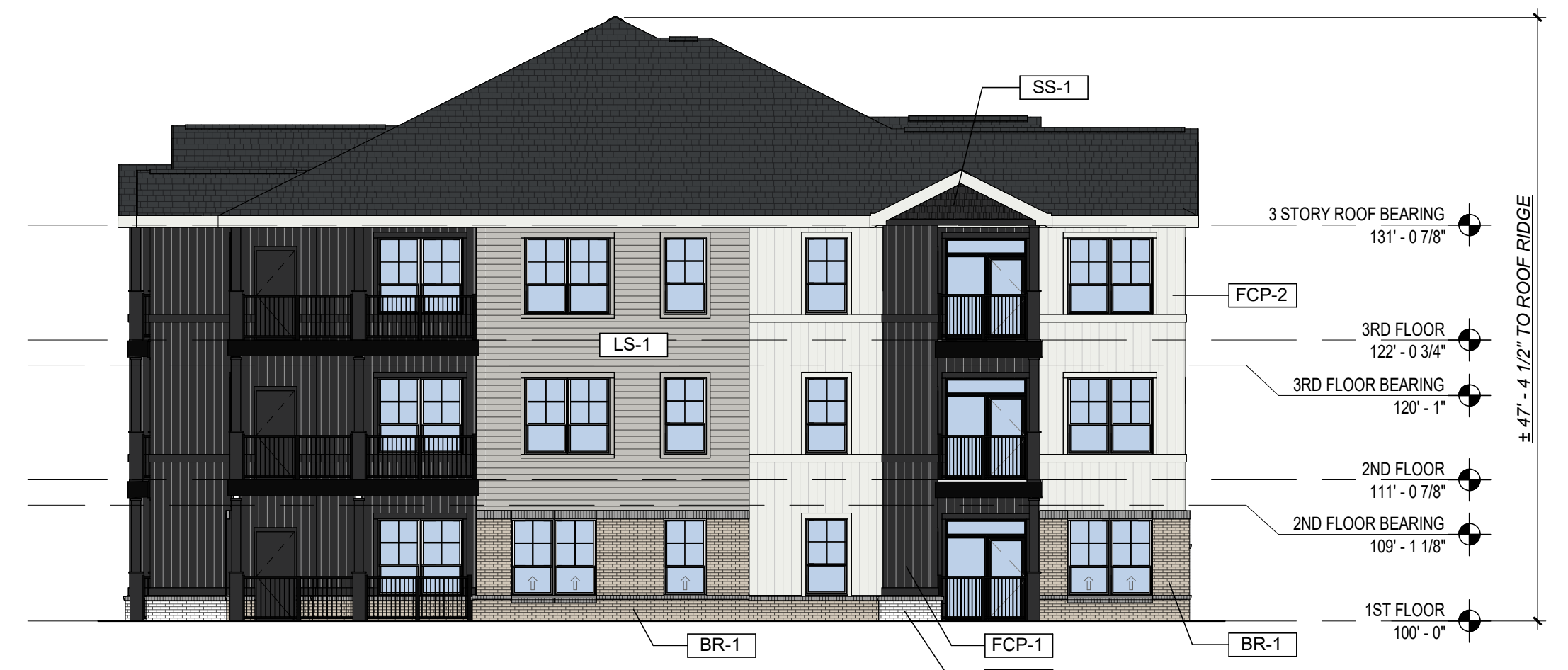
C A.20 Building 1 - side elevation 3/32" = 1'-0"
